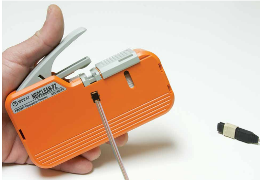
Placing PRIZM® LightTurn® connector into cleaner
